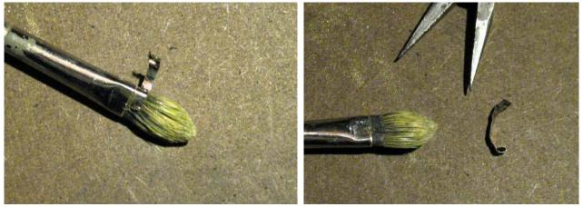
Carefully peel away a strip of metal with the cutters or a pair of needle nose pliers. (This strip can be sharp; use caution.) Use the file or fine sandpaper to deburr and smooth the new edge.
