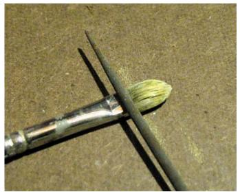
Using a fine metal file, score a line 1/8" back from the top of the ferrule, all the way round. It's not necessary to cut all the way through.
